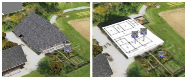
Figure 9. Normal view of the 3D building (left) and integration of construction plan as terrain texture (right)
