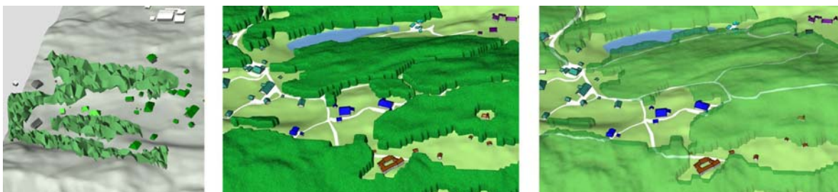
Figure 7: Woods: trees from digital surface model (left), block model (middle), transparent block model (right)
